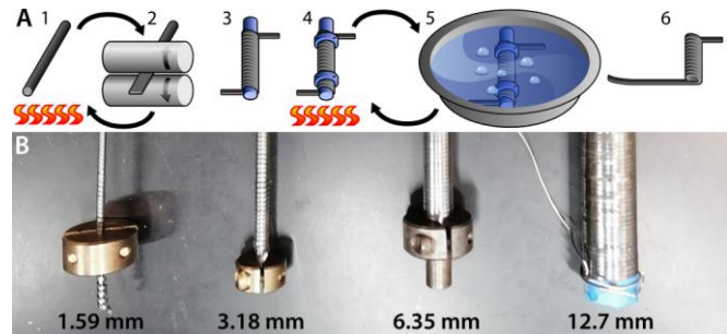
Figure 1. SMA ribbon actuator manufacture. (A) SMA wire is softened via annealing (1) and then flattened in a rolling mill (2), repeating these steps until desired thickness is reached; the flattened ribbon is wrapped around a steel rod (3), and clamped in place (4); the rod is heated and quenched (5), repeated three times; the ribbon is removed from the rod and unwrapped (6). (B) SMA ribbons prepared for programming by wrapping around steel rods of varying diameter and clamping in place.
